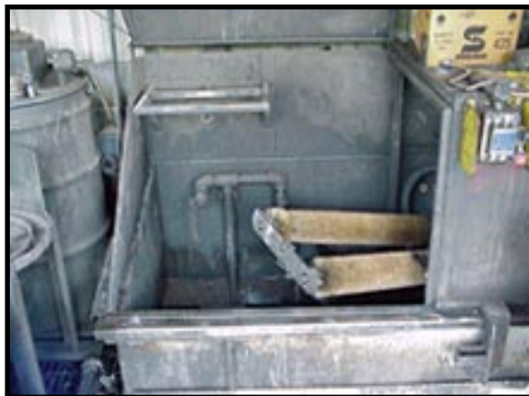
View of interior Drum Washer.
